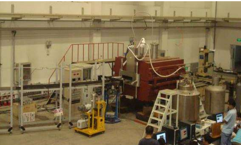
Superconducting dipole magnet, low temperature, power supply and measurement systems
