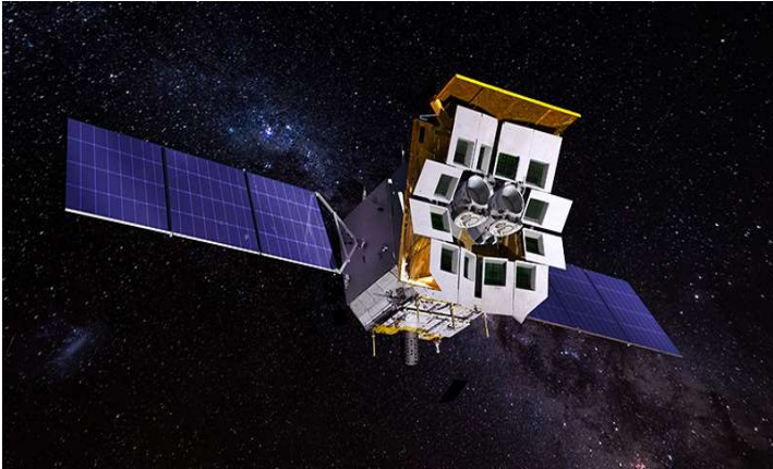
Einstein Probe satellite focal plane detector and X-ray telescope
