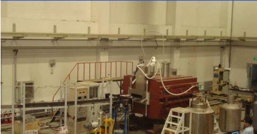
Superconducting dipole magnet, low temperature, power supply and measurement systems
